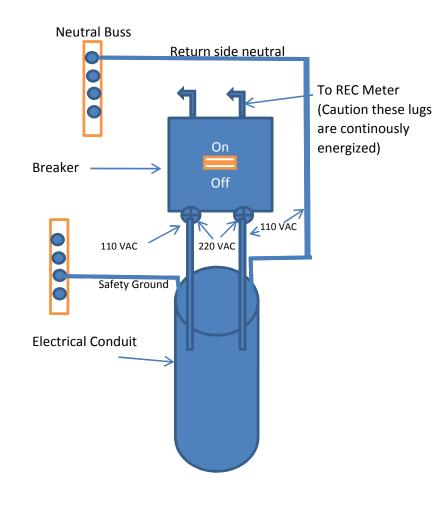
100 Amp - Use # 4 Copper or # 2 Aluminum 125 Amp - Use # 2 Copper or 1/0 Aluminum
